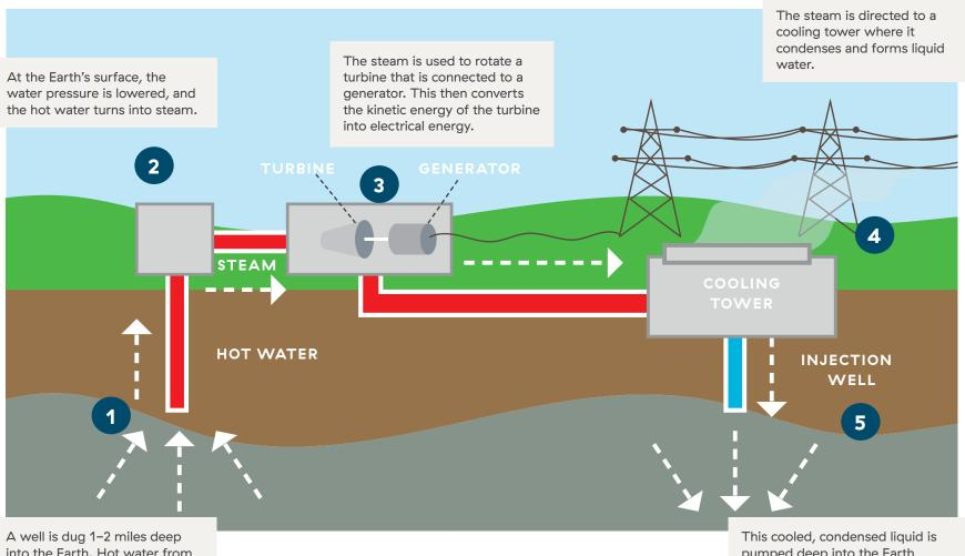
into the Earth. Hot water from deep underground is pumped to the Earth's surface under high pressure conditions. pumped deep into the Earth through another well. This allows the process to begin again.
